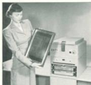
Material to be copied has been transferred directly to the developed plate.
