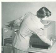
Charged Plate is now being exposed to original copy for a few seconds through the lens of the Camera.
