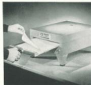
By placing paper master with transferred image in the Fuser for a few seconds, the print is made permanent.
