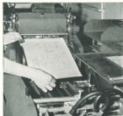
The processed offset paper master is placed in position on the cylinder of the duplicating machine and is ready to run.
