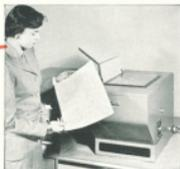
Material to be copied is placed face down on plate glass top of the Xerox Camera.
