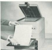
After development, the offset paper master is placed over the image on the plate.
